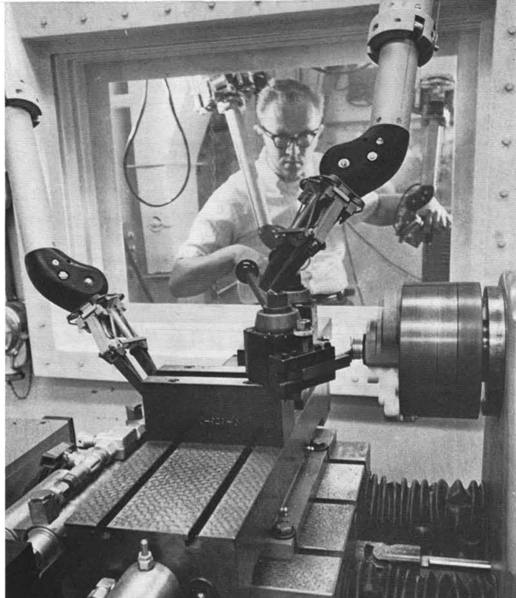
SAFETY was designed into this remote control facility in Bldg. 940 used for precision machining of explosive components and materials. Tom Massis demonstrates use of the master slave manipulators from control room. A small explosion in the chamber recently did negligible damage to equipment. Operator was completely protected by heavy shielding glass.
